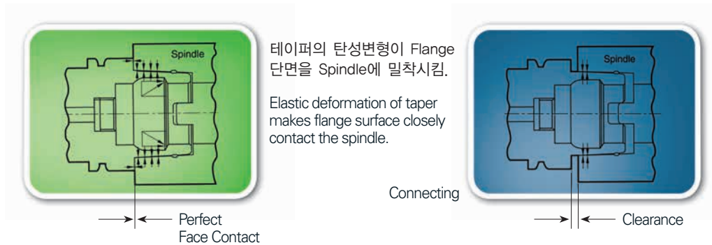
HSK shank -Perfect 2-surface constrained System
